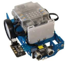
picture 13: mBot with display and accelerometer and gyro sensor
